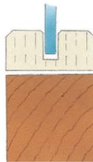
44mm wide Monolux channel on minimum 44mm wide softwood or hardwood frame. 1/2 hour fire resistance (stability & integrity)
