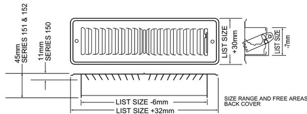
The 150 Series provides a range of supply and extract grilles and diffusers for floor, ceiling, sidewall and cill mounting. Fabricated from top quality 1.2mm mild steel the face louver blades are centrally split both right and left handed and set on an increasing angle deflection to provide a good discharge and spread of air.
