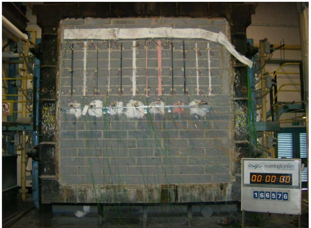
The unexposed face of the specimens after a test duration of 61 minutes
