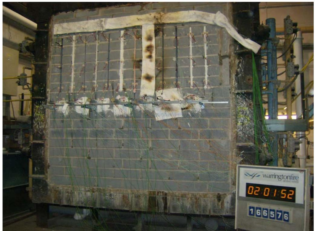
The unexposed face of the specimens after a test duration of 180 minutes
